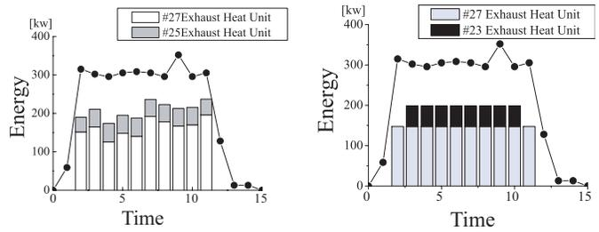
Fig. 16. The result of Machine Codes and Load Factors of Exhaust Heat Unit(left:GA, right:Expert)
