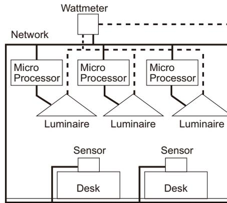
**Fig. 1.** Composition of the intelligent lighting system
