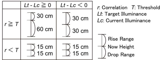
Fig. 2. One-time variation range of luminaire height
