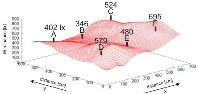
Fig. 5. Illuminance distribution (Using Intelligent Lighting System)
