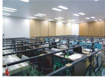
Fig. 7. Illuminance distribution measurement in Ecozzeria
